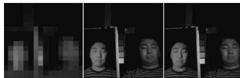
Figure 1. Left: A 16 \times 16 spectral image at 600nm. Center: The 512 \times 512 super resolution spectral image constructed by the proposed approach. Right: Ground truth (CAVE database [30]).
