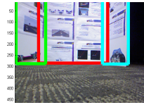
Figure 2: Detecting planes in 3D point cloud data collected using a Kinect. The population size is N = 167,028 and \theta = 30,000 . By setting P = 0.9 , on the 1 st level \varepsilon = 3 then r = 43 and on the 2 nd level \varepsilon = 100 then r = 714 .
