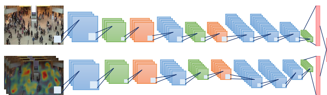
Figure 2: Deep model. The appearance and motion channels are input in two separate branches with the same deep architecture. Both branches consist of multiple layers of convolution (blue), max pooling (green), normalization (orange), and one fully-connected (red). The two branches then fuse together to one fully-connected layers (red).
