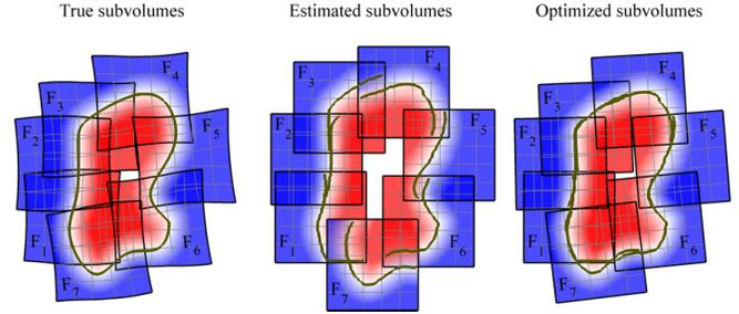
Figure 1: Locally-accumulated TSDFs (left) are shipped from GPU to host, effectively representing the *true* scene by a set of overlapping individually reconstructed subvolumes (center). Noise and drift are reduced by estimating an optimized 6-DOF pose for each subvolume (right).
