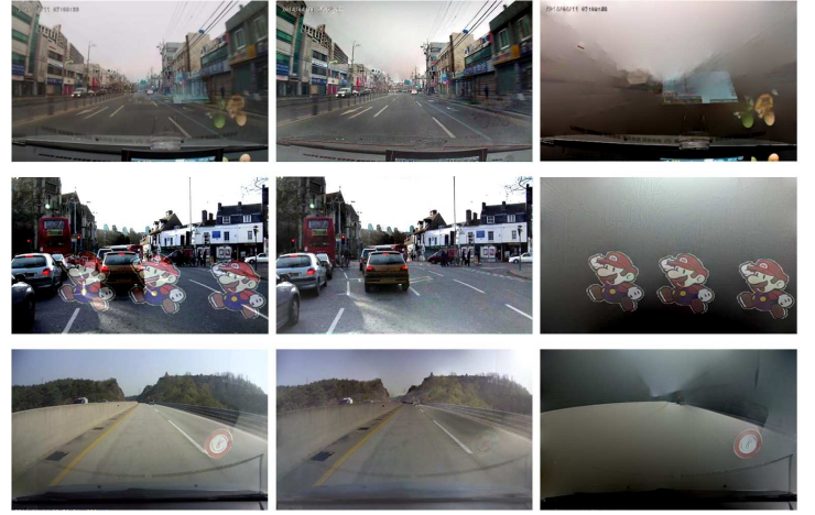
Figure 3: Frame results from three different videos. First, second, and third columns are input images, background layers, and reflection layers, respectively. The first and third rows are from real world black box videos, while the second row is from a synthetic video.
