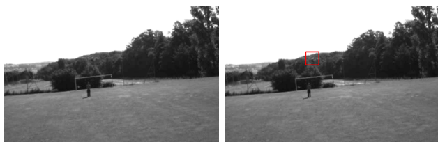
Figure 1: Detecting a small drone against a complex moving background. (Left) It is almost invisible to the human eye and hard to detect from a single image. (Right) Yet, our algorithm can find it by using motion clues.
