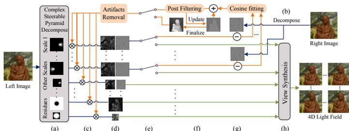
Figure 1: The pipeline of the whole proposed framework.
