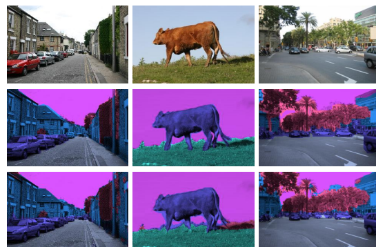
Figure 2: The results of scene labeling on the Stanford Background dataset. First row: input image; Second row: ground-truth; Third row: predicted image. Colors on images indicate labels — identical colors on ground-truth and predicted images indicate a correct labeling
