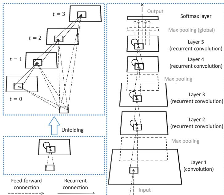
Figure 1: The overall architecture of RCNN. Left: An RCL is unfolded for  $T = 3$  time steps, leading to a feed-forward subnetwork with the largest depth of 4 and the smallest depth of 1. At  $t = 0$  only feed-forward computation takes place. Right: The RCNN used in this paper contains one convolutional layer, four RCLs, three max pooling layers and one softmax layer.
