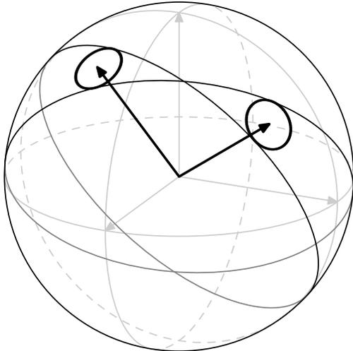
Figure 1: Epipolar geometry under translation.
