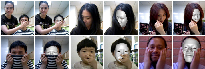
Figure 1: Calibration-free realtime facial performance capture on highly occluded subjects using an RGB-D sensor.
