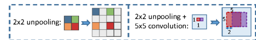
Figure 3: Illustration of unpooling (left) and unpooling+convolution (right) as used in the generative network.
