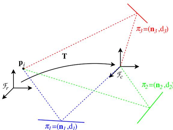
Figure 1: The geometry of the mirror-based camera pose estimation problem.
