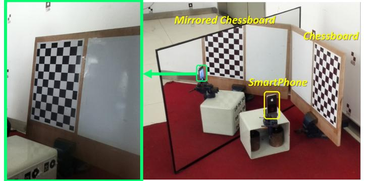
Figure 2: Extrinsic calibration of a smart phone's camera-pair: Both front and back camera can see the chessboard only via mirror reflections. We apply our mirror based pose estimation to find both cameras' absolute pose with respect to the calibration target given only (at least 3) mirrored views of the object. By combining the absolute poses, we can then easily retrieve the relative pose between the non-overlapping pair of cameras.
