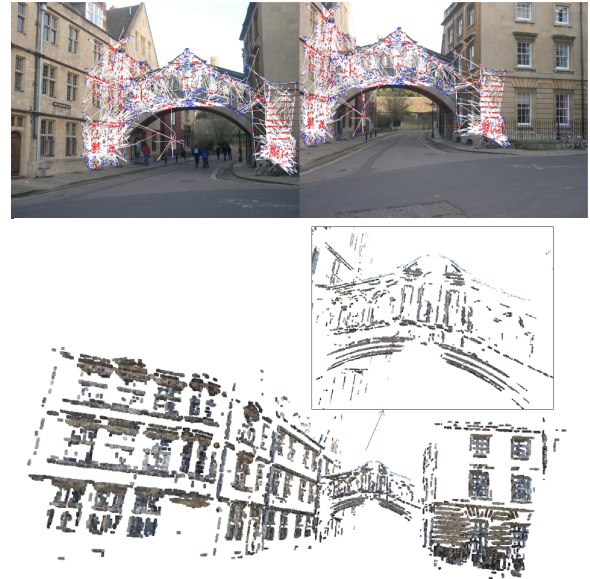
Figure 3: Top: We consider pairs of keypoint correspondences (shown in blue) to form virtual lines (white) to identify several hundreds of additional point matches (shown in red). Bottom: We show line-based 3D reconstruction of the Bridge of Sighs in Oxford.
