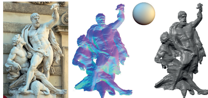
Figure 1: (left) Pipeline for training and testing. For each test image, we estimate a reflectance map to train the regression forests on synthetically generated data. We optionally enforce integrability on their pixel-wise predictions. (right) Qualitative results for shape and reflectance estimation from a single internet image: input image [9], estimated normals and reflectance map, and novel view (from left to right).
