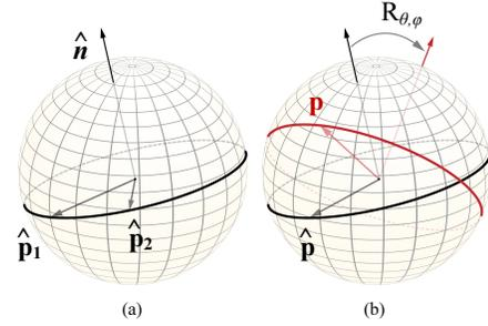
Figure 2: Left:  $\hat{\mathbf{p}}_1$  and  $\hat{\mathbf{p}}_2$  are two end points of a geodesic line segment before warping. Right:  $\hat{\mathbf{p}} = \hat{\mathbf{B}}\mathbf{s}$  is a shifted point on the same plane (black) as  $\hat{\mathbf{p}}_1$  and  $\hat{\mathbf{p}}_2$ . This plane is rotated by  $\mathbf{R}_{\theta, \phi}$  and mapped to another plane (red). Then  $\hat{\mathbf{p}}$  becomes  $\mathbf{p}$  after warping.
