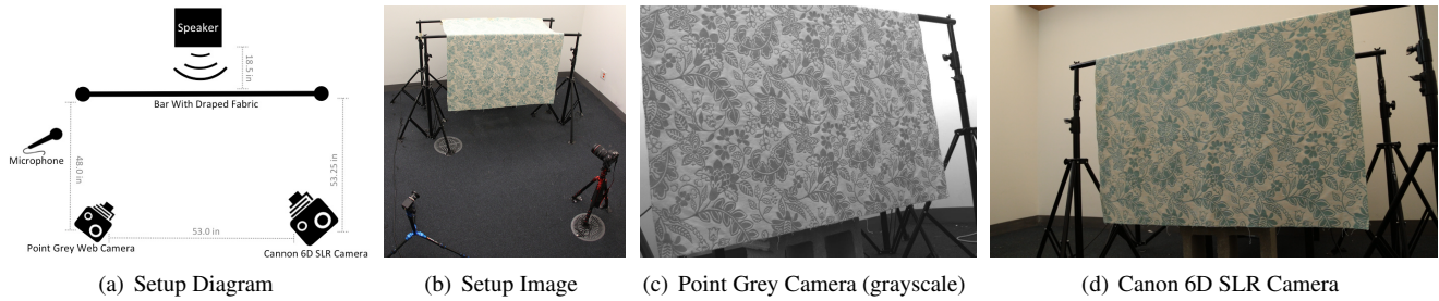
Figure 5. Videos were recorded of the fabric moving from (c) a grayscale Point Grey camera ( 800 \times 600 pixel resolution) at 60 fps and (d) an RGB SLR Camera (Canon 6D, 1920 \times 1080 pixel resolution) at 30 fps. The experimental layout (a,b) consisted of the two cameras observing the fabric from different points of view.
