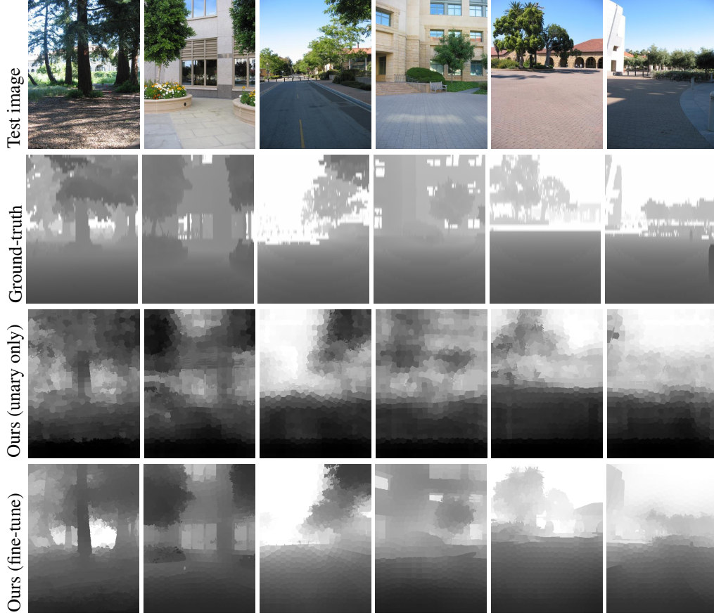
Figure 4: Examples of depth predictions on the Make3D dataset (Best viewed on screen). The unary only model gives rather coarse predictions, with blurry boundaries and segments. In contrast, our full model with pairwise smoothness yields much better predictions.
