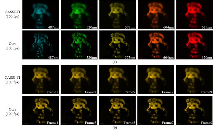
Figure 2: HSHS video reconstruction results of a fast moving doll under ordinary indoor illumination. Exposure time for CASSI and PanCam is 100ms and 10ms, respectively. (a) Results of different selected bands at one temporal location. (b) Results of one selected band at different temporal locations. CASSI-TI denotes the temporal interpolation of CASSI reconstruction.
