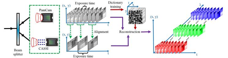
Figure 1: Data flow in the proposed dual-camera system.
