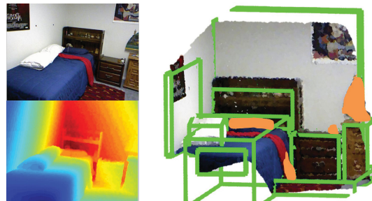
Figure 1: With a given RGBD image (left column), our method explores the 3D structures in an indoor scene and estimates their geometry using cuboids (right image). It also identifies cluttered/unorganized regions in a scene (shown in orange) which can be of interest for tasks such as robot grasping.
