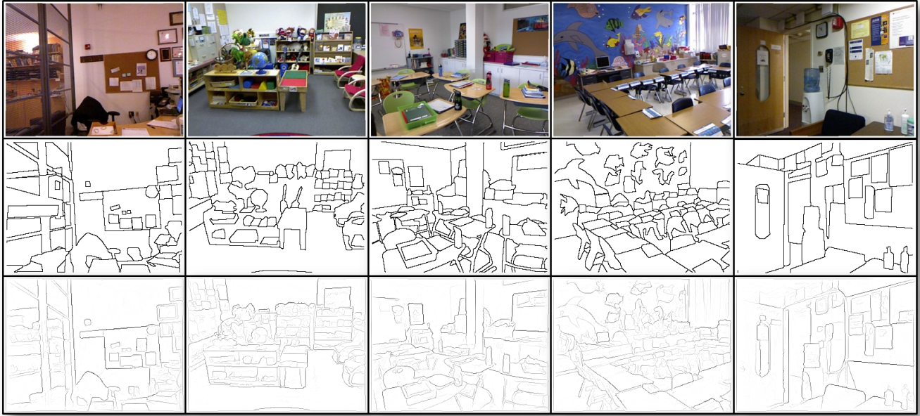
Figure 6. Illustration of our contour detection results on the NYUD dataset [43] for five selected example images (Depth images are not used). In each example, we see the original image and the ground truth and our results, respectively. Although our deep contour features are learned from the BSDS dataset, they can represent the object contours in NYUD dataset well.
