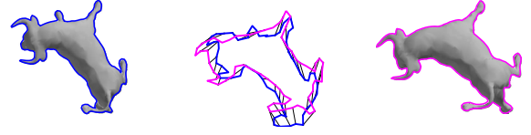
Figure 4: Contour Dissimilarity Measure. The black lines connecting the blue and pink contours connect between similar points along the contours. The average spatial distance is then computed and later scaled accordingly. The computed distance between the two shapes illustrated above is 20.6^\circ , and the true geodesic distance is in fact 23.5^\circ .
