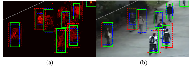
Figure 7. (a) Estimating bounding boxes from the density map. The estimated box is green, the prior box is dashed-red, and the estimated box without using prior information is dashed-blue. (b) The corresponding image.
