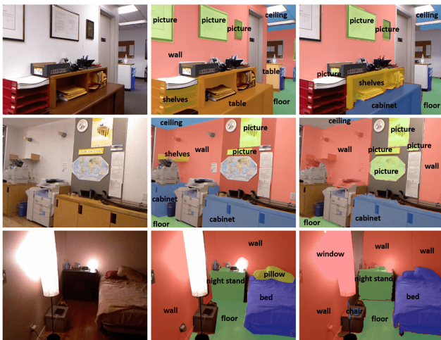
Figure 4. Sample semantic segmentations generated by our system. Left to right: RGB image, ground truth semantic segmentation, our segmentation.
