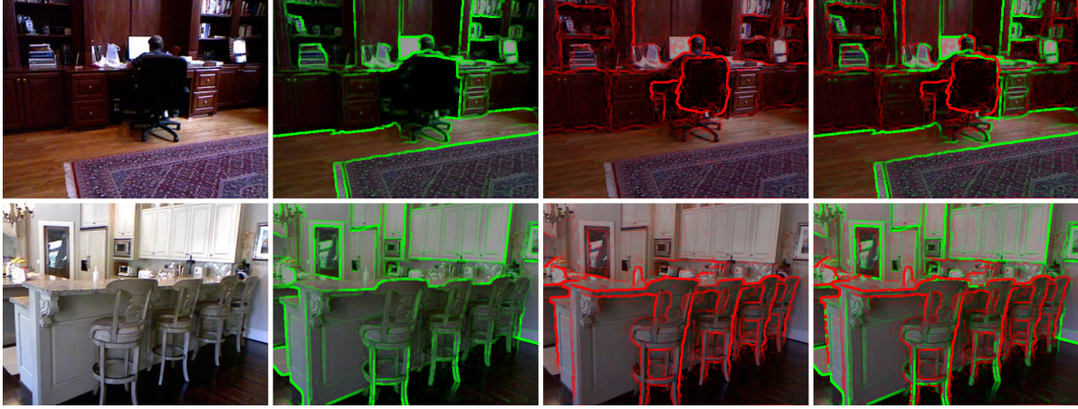
Figure 2. Depth and intensity boundary complement each other. Left to right: original image, boundaries extracted from the intensity image, boundaries extracted from the depth image, boundaries resulting from the fusion of RGB and depth information, cf (2) with winning channel shown.
