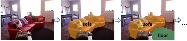
Figure 3. Sequential Search-Based Structured Prediction procedure at test-time. We iteratively apply the learned policy and select the action predicted as most suitable given current state.
