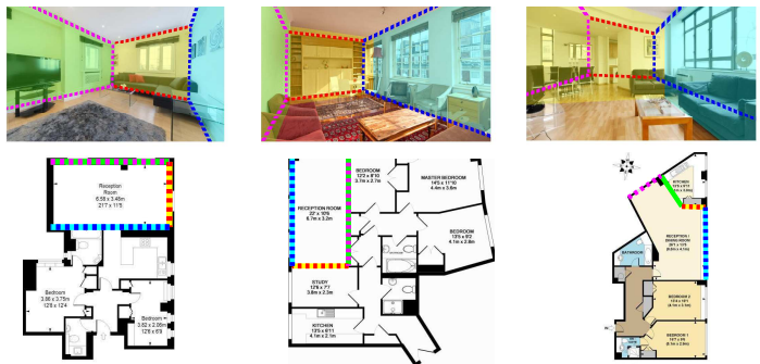
Figure 2: Room layout estimation and wall alignment with our model. Top row show the estimated vertical walls (solid color), and GT layout (dashed lines). Bottom row shows the floor plans with predicted and GT alignments. Solid colors show alignment predicted by the model, where the yellow solid line denotes the front wall. GT alignment is shown with dashed lines.
