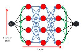
Figure 6. The spatio-temporal graph to extract multiple objects is highlighted here. The bounding boxes in each frame are shown as red circles. The temporal costs shown as blue directed edges indicate inter-frame costs to connect a path through two bounding boxes in successive frames. The intra-frame spatial costs are indicated as green undirected edges. They penalize extraction of the same object in multiple paths. Best viewed in color.
