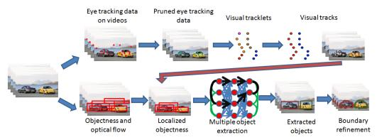
Figure 3. Block diagram of the proposed approach to extract multiple objects from videos using eye tracking prior. The top row indicates the eye tracking processing stage. The bottom row is the multiple object extraction framework guided by the visual tracks. Best viewed in color.
