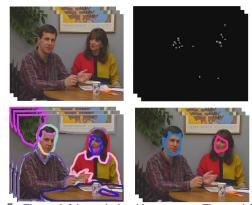
Figure 7. The top-left image is the video sequence. The top-right shows eye tracking samples in a frame from the sequence. The bottom-left figure highlights the exhaustive manual object annotations in the scene. Finally, the bottom-right illustrates the important ground truth objects which attract visual attention obtained according to Section 4.1. Best viewed in color.
