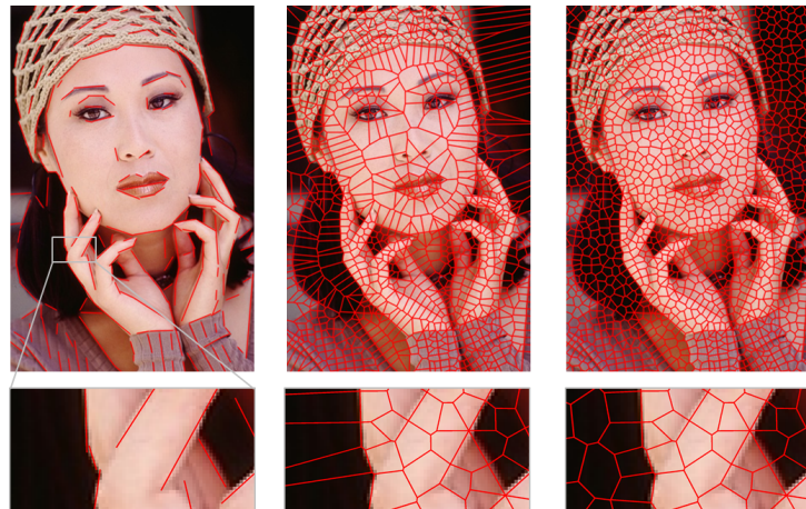
Figure 2: Overview. Left: line-segments are first extracted from the input image, and consolidated to bring spatial coherence. Middle: an initial Voronoi partition that preserves the line-segments and their junctions is then created by inserting anchors at some specific locations. Right: the Voronoi partition is homogenized by point process.
