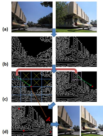
Figure 1: (a) Reference (left) and target (right) images, (b) edge maps of (a), (c) patch matching and sliding window, (d) left: target center voting in edge maps, right: image cropping with the same center.
