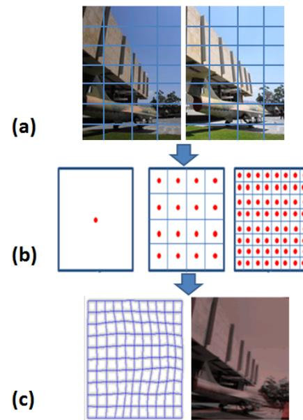
Figure 2: (a) Initial global affine estimation and image partitioning. (b) Hierarchal block partitioning for coarse-to-fine local affine estimation. (c) Image registration result.
