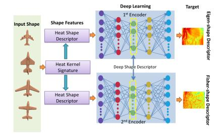
Figure 2: Pipeline of learning deep shape descriptor. Given input shapes, three steps are included along with the pipeline: 1)Heat kernel signatures are extracted for each shape in the database. Heat shape descriptor are computed based on HKS. 2) Heat shape descriptors are fed into two deep neural networks with target values using ESD and FSD, respectively. 3)The deep shape descriptor is formed by concatenating nodes in hidden layer (circled by yellow dash lines).
