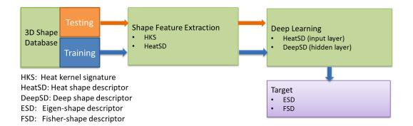
Figure 1: Main components of the proposed method.
