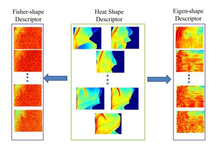
Figure 4: Pipeline of generating Eigen-shape descriptor and Fisher-shape descriptor. A collection of Heat shape descriptors are used to train Principal Component Analysis (PCA) and Linear Discriminant Analysis (LDA). The trained Eigen-shape descriptors are illustrated on the right and Fisher-shape descriptors are shown on the left.
