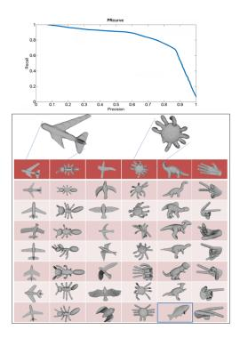
Figure 7: **Top**: Precision-Recall plot shape retrieval performance on incomplete models. **Bottom**: partial shape retrieval. The models shown in the first row are partial and incomplete models. Each column represents the retrieval result using the 3D model in the first row of each column as the query model. Top 7 retrieval results are listed in the figure.
