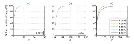
Figure 2. PCA accumulative energy of the responses in each layer, presented as the sum of largest d' eigenvalues (relative to the total energy when d' = d). Here the filter number d is 96 for Conv1, 256 for Conv2, and 512 for Conv3-7 (detailed in Table 1).
