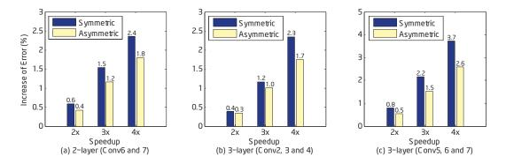
Figure 5. **Symmetric vs. Asymmetric**: the cases of 2-layer and 3-layer approximation. The speedup is computed by the complexity of the layers approximated. (a) Approximation of Conv6 & 7. (b) Approximation of Conv2, 3 & 4. (c) Approximation of Conv5, 6 & 7.
