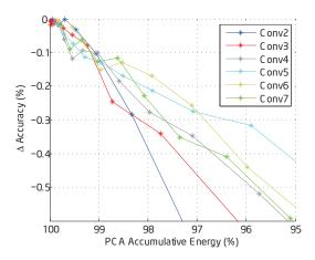
Figure 3. PCA accumulative energy and the accuracy rates (top-5). Here the accuracy is evaluated using the linear solution (the nonlinear solution has a similar trend). Each layer is evaluated independently, with other layers not approximated. The accuracy is shown as the difference to no approximation.
