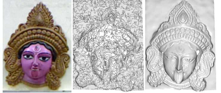
Figure 1: Refined depth map estimates of a painted terracotta plaque of Kali using our approach.
