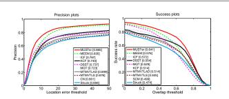
Figure 2: Quantitative comparison in CVPR2013 OOTB. The performance score for each tracker is shown in the legend. For each figure, only the top 10 trackers are presented.
