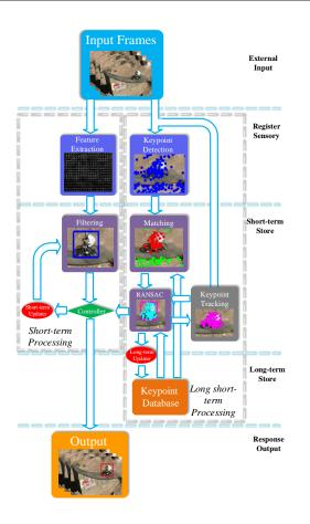
Figure 1: A system flowchart of the proposed tracker based on the Atkinson-Shiffrin Memory Model.
