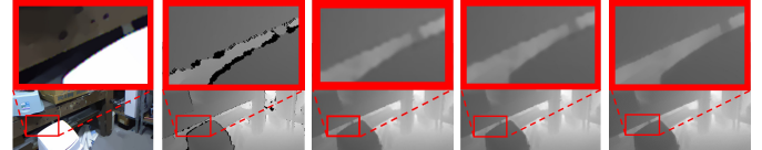
L_0 -RGB Raw depth 1st level 2nd level 3rd level Figure 4. Multi-scale refinement of the depth map. 1st: coarsest level; 2nd: middle level; 3rd: finest level. For illustration, the depth maps in the 1st and 2nd levels are bicubic upsampled to the resolution of the 3rd level.
