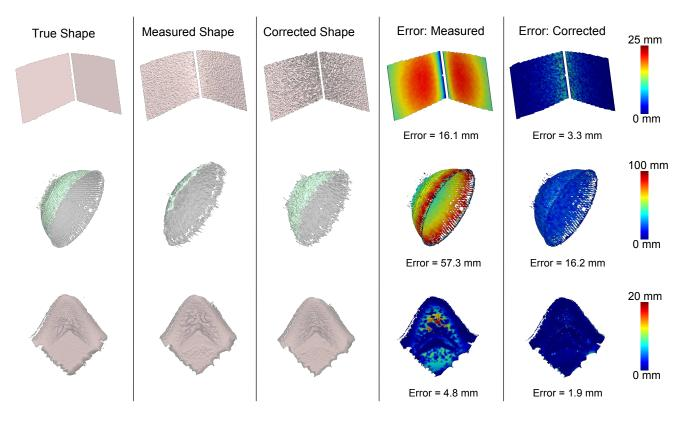
Figure 3. Our MPI correction algorithm reduces the root mean squared error on a variety of objects (simulated experiments). The first column shows the ground truth point cloud for a given object. The second column depicts the measured point cloud, simulated using rendering software. The output of our algorithm is shown in the third column. Finally, error comparisons with ground truth are shown in the fourth and fifth columns.
