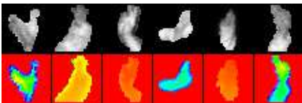
Figure 3. Successes and failures of the DFE classifier: Pairs of depth+IR images are presented, where the top row shows the IR images and the bottom the depth images in every pair. The 3 pairs on the left show successfully classified pairs for the 3 hand shape classes considered (Open, Closed, Lasso). The pairs on the right show miss-classification errors (false negatives).
