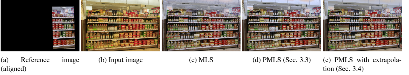
Figure 3: MLS vs. PMLS. Matching errors adversely affect the performance of the MLS algorithm, while the PMLS can absorb the matching errors due to the probabilistic modeling (d). Color transfer in the non-overlapping region is also effectively modeled with our extrapolation scheme (e). We recommend the readers to zoom-in to see the difference clearly.
