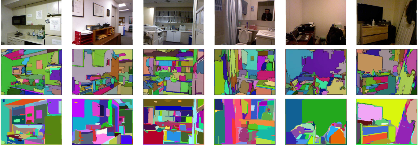
Figure 6. Segmentation results from different 3D RGBD scenes from the NYU data set[18]. The top row is the images, the 2nd row is the hierarchical result only using color with a hierarchical level of 0.7 described in [7], and the bottom row is our approach with a hierarchical level of 0.7.
