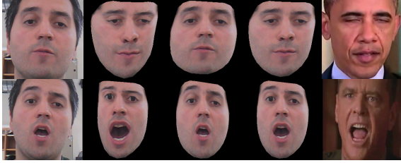
Figure 3. Comparison of warping approaches. Left: Selected user frame. Right: Target pose. Middle left to right: non-rigid warping (Eq. (5)), affine warping (Eq. (6)), and our approach (Eq. (7)).
