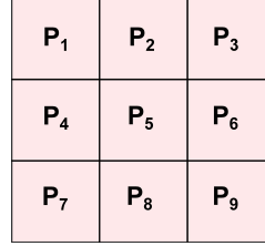
Figure 1. Geometric interpretation of the differential operator \delta_i at vertex i = 5 . It measures the deviation between x_5 and its center of mass \frac{1}{d_5} \sum_{j \in N(5)} w_{ij} x_j .
