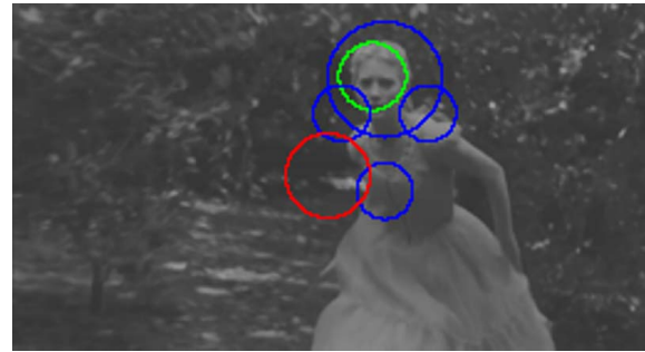
Figure 3. Semantic candidates. The center candidate is red, green ellipses are faces, and blue are human body candidates. Since the body is large it is represented by four candidates. These candidates cover most of the semantically salient regions in the frame.
