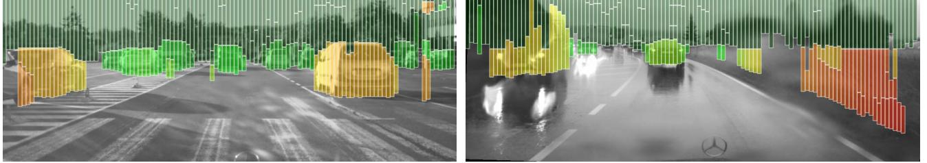
Figure 6: Results of our extensions to the Stixel computation of Pfeiffer *et al.* The difference to Figure 5 is striking. Using stereo confidence cues in the sensor model allows to remove nearly all false positives while the detection rate is kept high.
