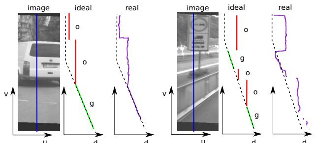
Figure 4: The blue line marks the column for segmentation. Red and green denote the ideal segmentation into object and ground. The dashed line is the expected ground profile and the disparity measurement vector is marked using purple.
