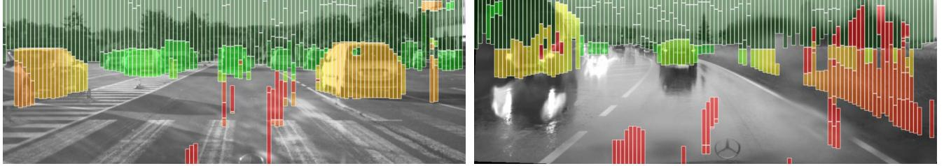
Figure 5: Stixel results for two visually challenging situations are using the approach of Pfeiffer *et al.* One can clearly see numerous false positives (mostly red) on the ground surface caused by stereo matching.
