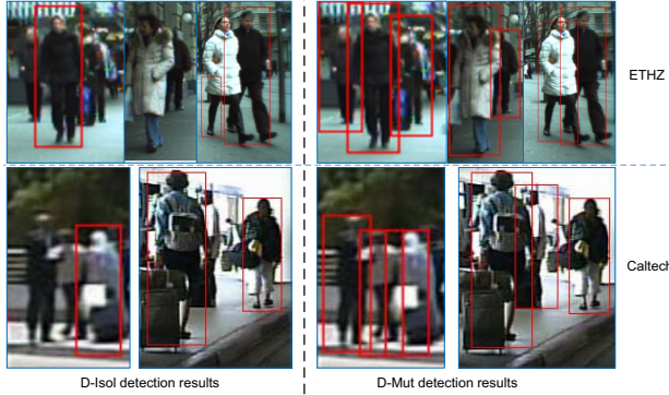
Figure 8. Detection results comparison of D-Isol and D-Mut on the Caltech-Train dataset and the ETH dataset. All results are obtained at 1 FPPI.
