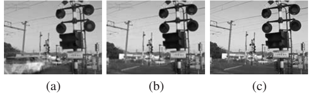
Figure 8. Background subtraction by (a) K-SVD [2] (b) batch robust dictionary update, and (c) our method with online dictionary update. Our results do not contain the “ghost” artifacts, similar to those produced by batch dictionary learning.
