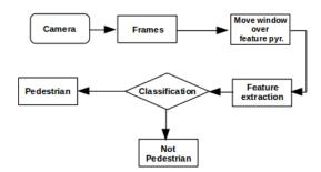
Figure 2. Architecture of the pedestrian detection module.
