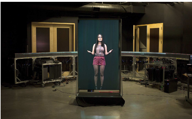
Figure 9. Photograph of subject shown on the automultiscopic projector array.
