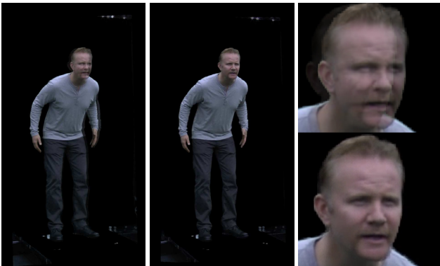
Figure 6. (left) View generated using bilinear interpolation exhibits aliasing. (center) View generated using optical flow interpolation has sharper edges and less aliasing. (right) Closeups of face.
