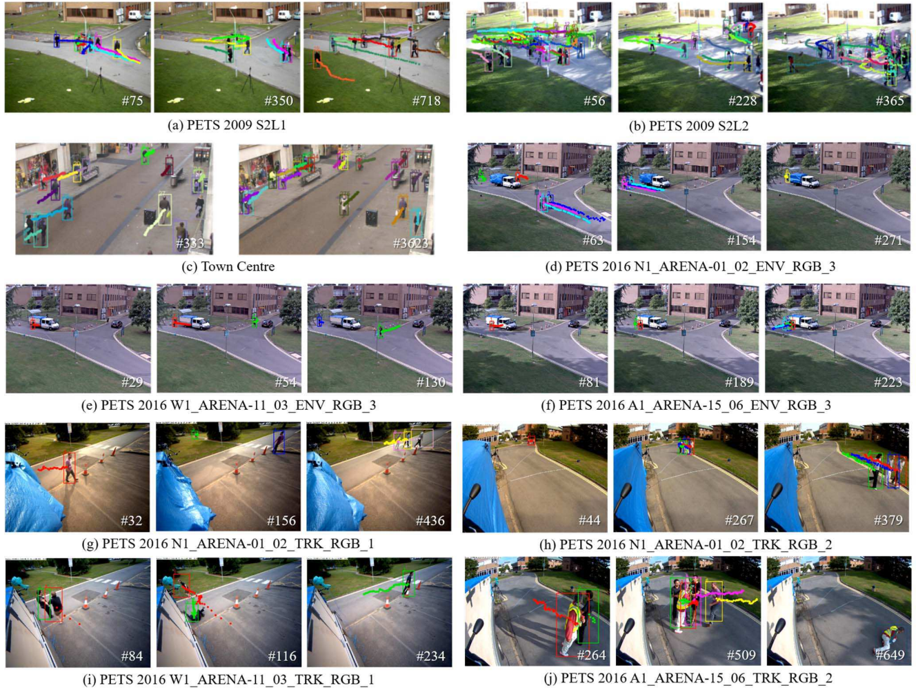
Figure 9. Tracking results of the proposed method for each dataset. At each frame, bounding boxes, recent trajectories (50 frames), and IDs of tracks are illustrated in color boxes, lines, and numbers.
