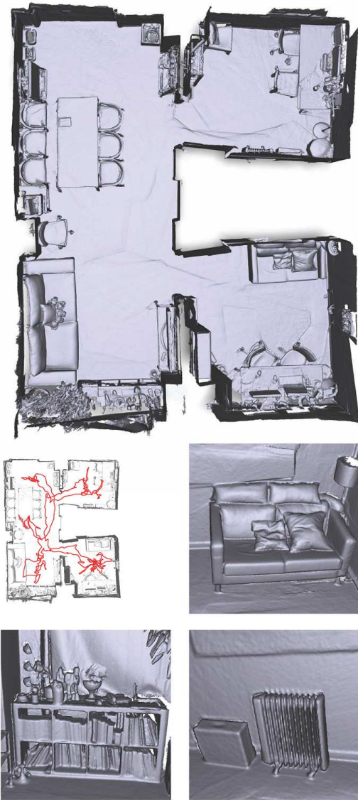
Figure 1. Automatic online reconstruction from a sequence of handheld RGB-D images. The top shows the reconstructed 3D model of our two-pass system. The middle shows our optimized camera trajectory and the rest show some details of the model. The area of this scene is about 40m^2 and the camera trajectory is about 79 meters long. Scanning the room takes about 360 seconds and the online reconstruction finishes within 170 seconds, i.e. 170 seconds after the user terminates the scanning process.
