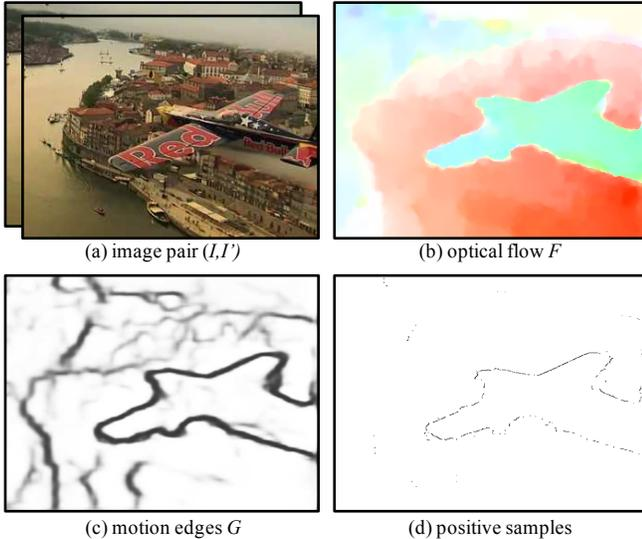
Figure 3. Illustration of motion edge detection. (a) Input images. (b) Colorized EpicFlow results  $F$  on the input images. (c) Motion edges  $G$  computed by applying an edge detector  $\mathcal{E}$  to the colorized flow. (d) Motion edges  $G$  after alignment, non-maximum suppression, and aggressive thresholding. The aligned motion edge map  $G$  serves as a supervisory signal for training an edge detector.
