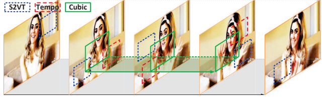
Figure 4: Illustration of three cropping schemes. S2VT crops patches from random locations across all frames in a sequence. The Tempo also crops patches from random locations, but from a randomly cropped subsequence. The Cubic crops patches from a random location shared across a randomly cropped subsequence.
