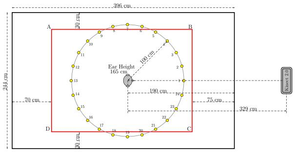
Figure 5. Setup for data recordings. The 24 highlighted dots in a circle labels the positions used to model the relationship between different input angles and the exhibited audio features.
