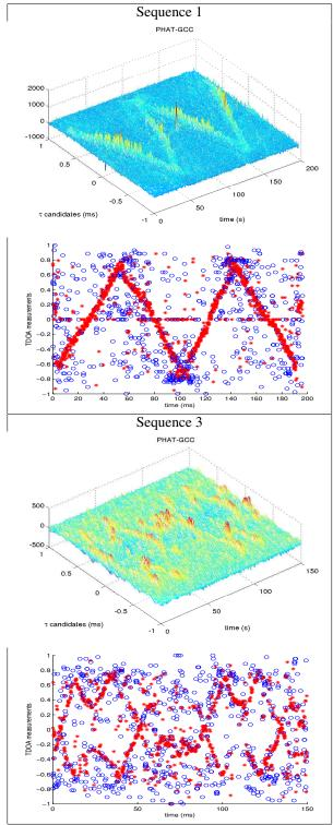
Figure 6. PHAT-GCC results and detected TDOAs from Sequence 1 and Sequence 3. The red-starred points denote the first peak-related TDOA while the blue circles represent the second one. The peaks in Sequence 1 are very smooth, which clearly exhibits the speaker's trajectory. However, despite some peaks being related to the real positions in Sequence 3, many more false alarms are obtained.
