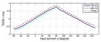
Figure 3. Illustration of the relationship between the resultant TDOA  $\tau$  with the azimuth  $\alpha$ . This was trained from off-line recordings at 16 kHz and 48 kHz. The third-order polynomial curve fitting is applied to model the audio likelihood function. We lifted the curve at 48 kHz, and lowered the fitted curve via a shift of 0.1 either way to improve visualization.
